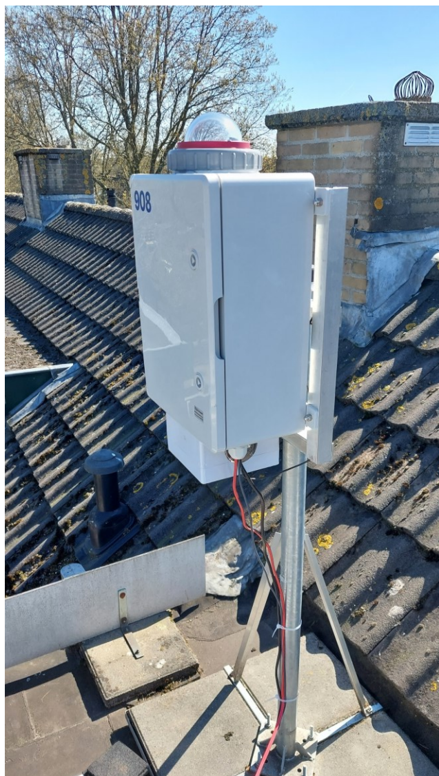
Figure 3 – A new box for the all-sky camera EN908 Ermelo. A plastic dome is protecting the lens against dew and rain.
