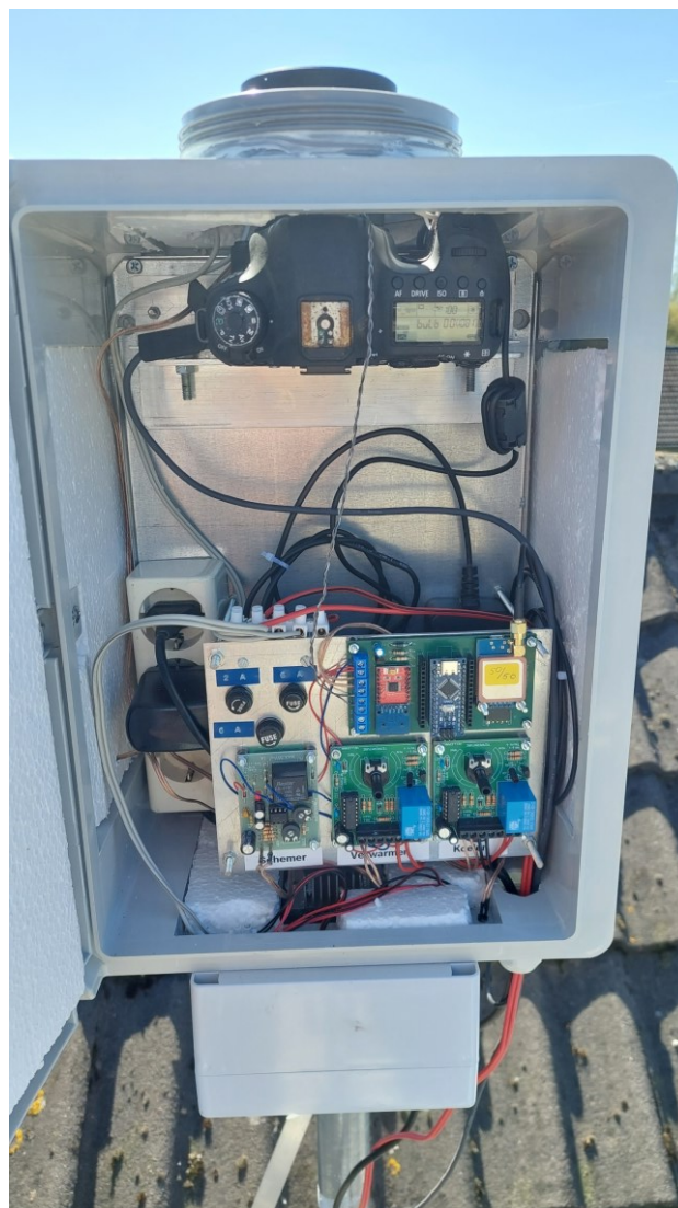
Figure 4 – Inside of the new all-sky housing EN908 Ermelo. During periods without rain the camera can operate without the plastic dome. This gives much better measuring results, especially with fireballs appearing low above the horizon.
