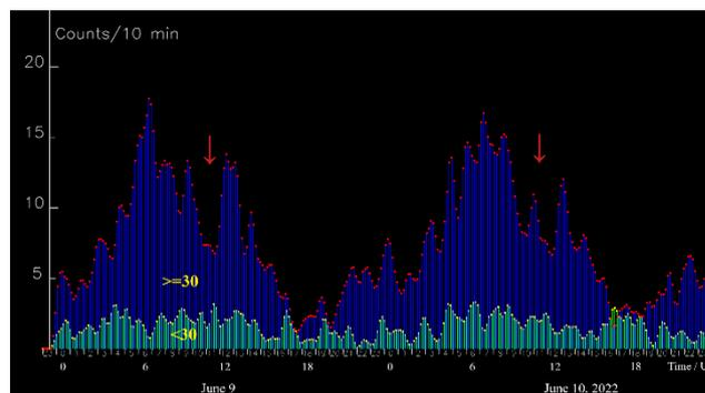
Figure 6 – Meteor detection rate for small echoes (< 30 pixel) and large ones ( $\geq 30$  to 100k pixels). Only the rate of large echoes exhibits dips. No notch is observed in the detection rate of small echoes at the dip. The data are from the left hand circularly polarized antenna.
