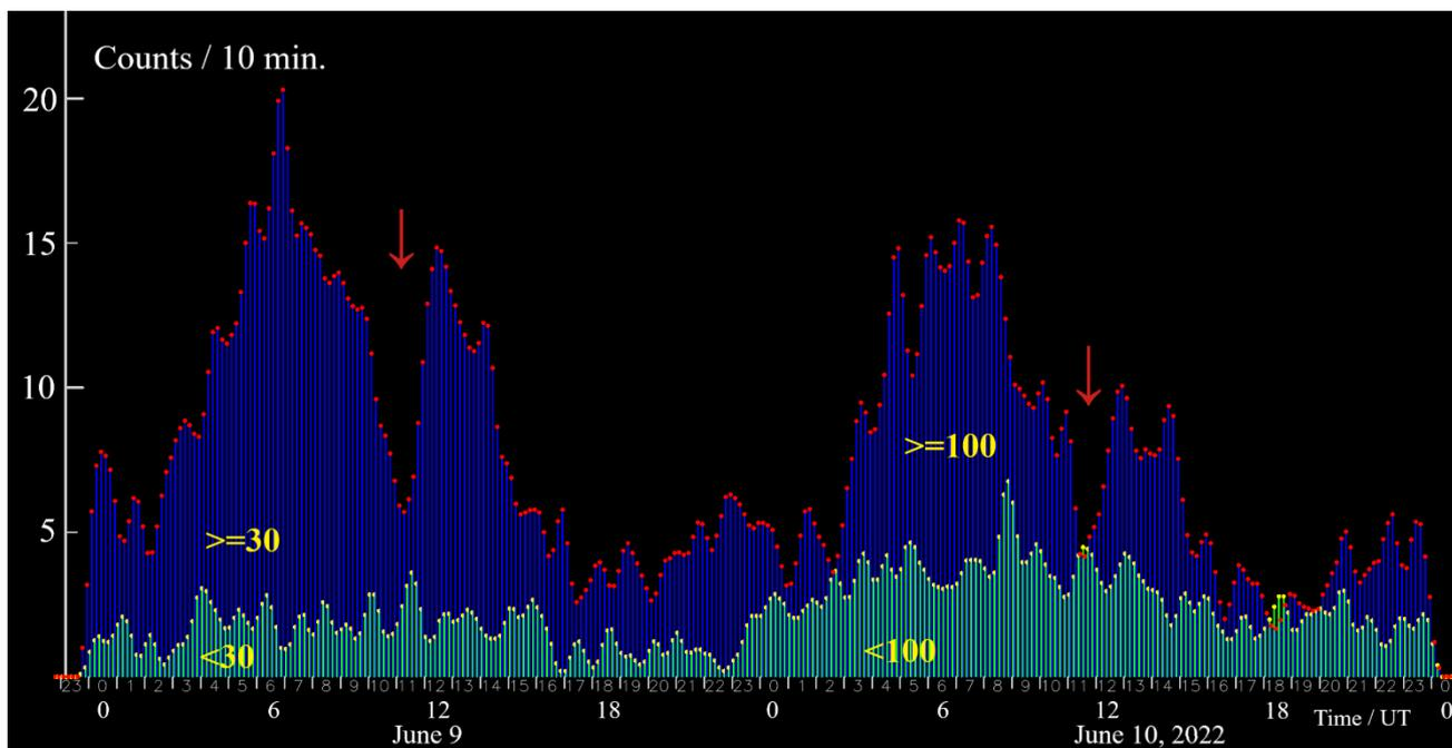
Figure 7 – Meteor detection rate for small echoes (< 30 or < 100 pixel) and large ones ( $\geq 30$  or  $\geq 100$  to 100k pixels). The data are from the right hand circularly polarized antenna. The small echoes show an increase at the notch, see text. Basically, it makes no difference whether the threshold is 30 or 100 pixel.
