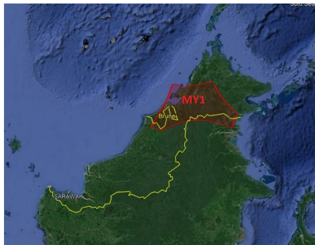
Figure 14 – GMN camera field intersected at 100 km elevation, for the first camera installed in Malaysia. The letter code refers to the camera ID, e.g., 1 = MY0001.
