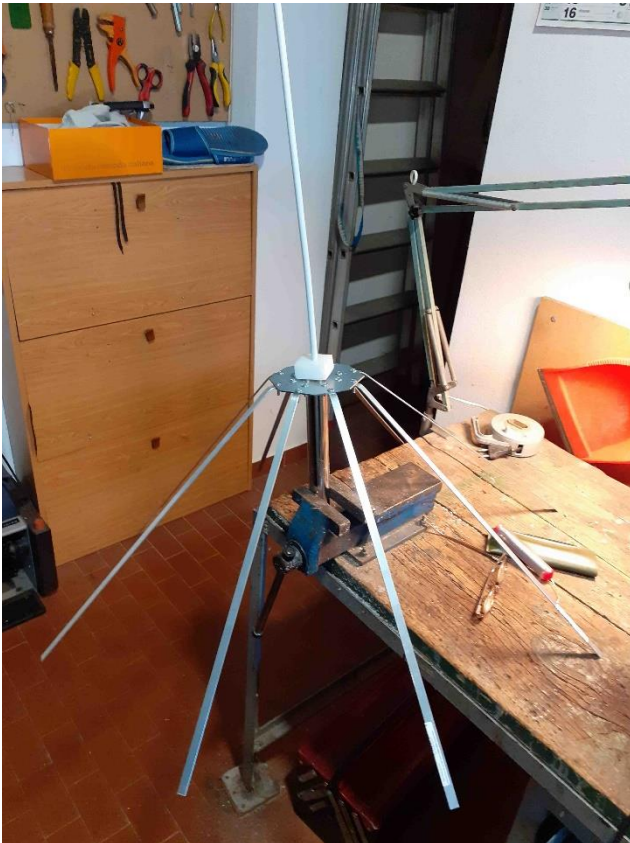
Figure 15 – Self-built ground plane antenna “Carmelina_143”.
