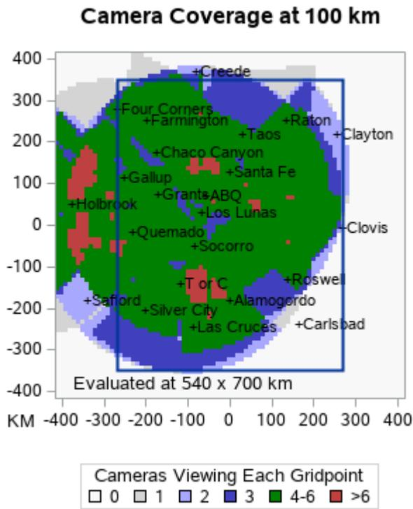
Figure 7 – Coverage at 100 km by the NMMA and the Lowell network after optimization.
