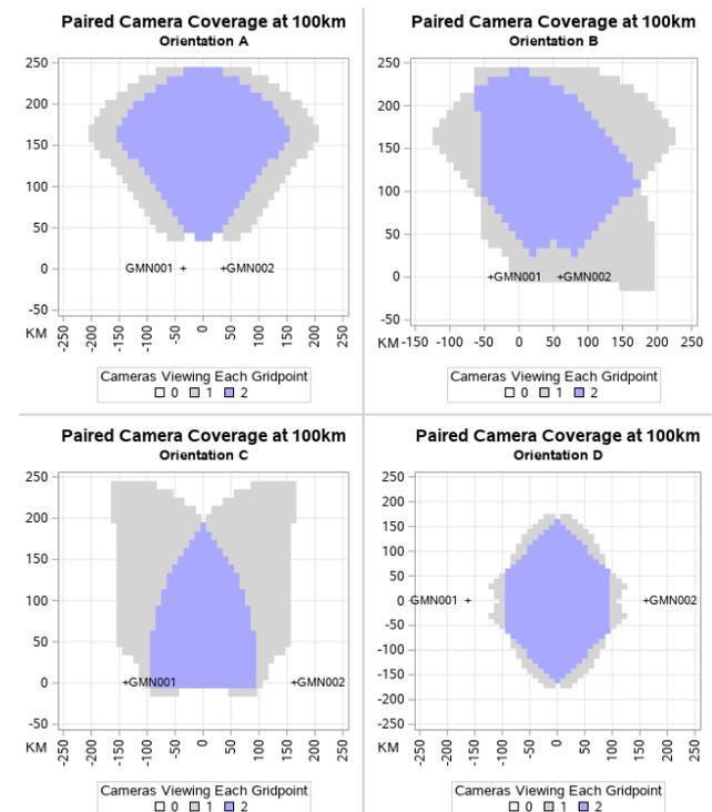
Figure 2 – Four possible camera orientations for a two-station network. For Orientation A, GMN001 & GMN002 are both aimed perpendicular to the line between the two stations. For Orientation B, GMN001 is oriented perpendicular to the line whereas GMN002 is at a 45° angle toward GMN001. For Orientation C, each camera is oriented at a 45° angle towards each other. For Orientation D, the two cameras are aimed toward each other.
