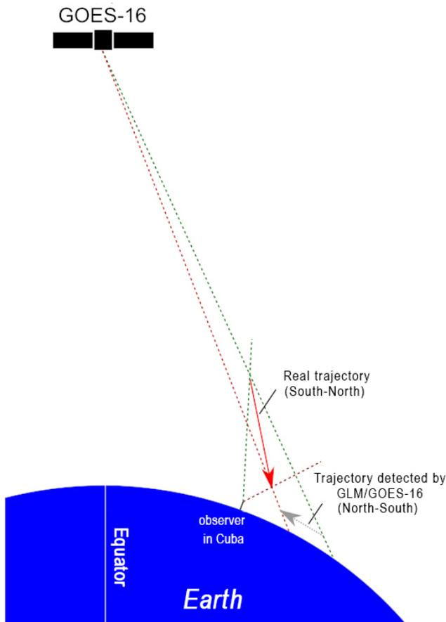
Figure 3 – How the parallax difference can interfere with the direction of the bolide detected by GOES-16. The green lines are the direction of the bolide detected by GOES-16. The red lines are the directions of the end point.
