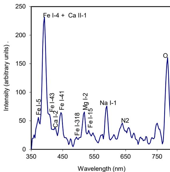
Figure 14 – Calibrated emission spectrum of the SWEMN20210812\_215832 fireball.
