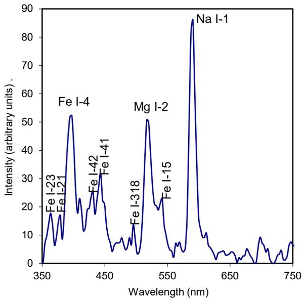
Figure 18 – Calibrated emission spectrum of the SWEMN20210818\_002016 fireball.
