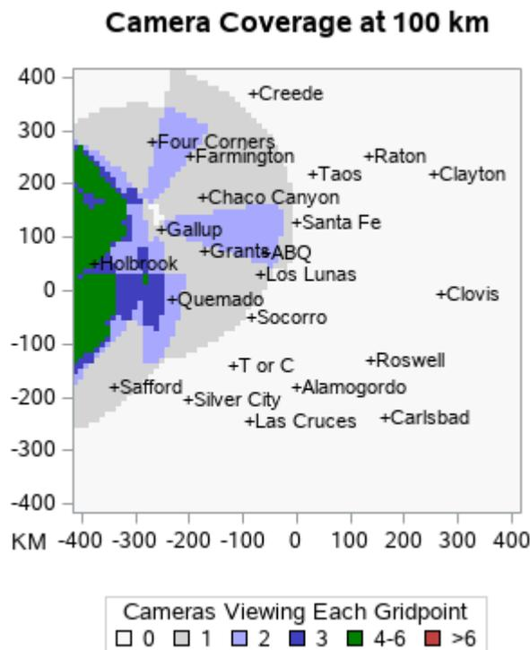
*Figure 5* – Extension of coverage at 100 km by the Lowell Network into New Mexico.
