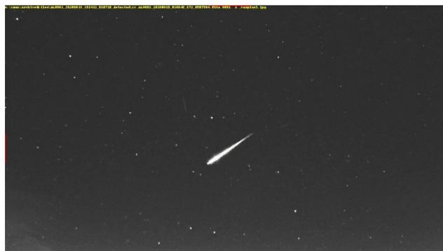
*Figure 6* – An example of a meteor picture obtained with an RMS camera with a f/0.95, 3.6 mm lens (BE0001, Grapfontaine). Notice the number of stars visible compared to the typical poor images obtained by Watecs.
