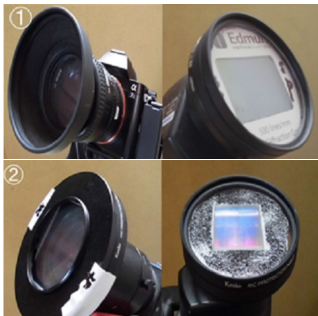
Figure 1 – Transmission type diffraction grating film with 500 lines per mm, 5 units (Top), transmission blazed diffraction grating with 600 lines per mm, 2 units (Bottom).
