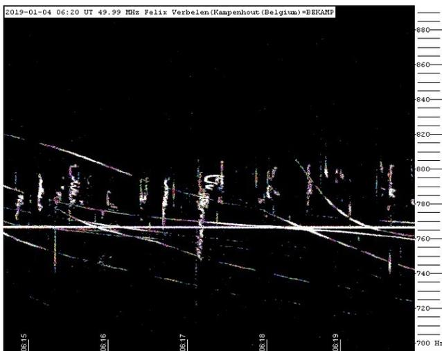
Figure 5 – A 5-minutes SpecLab picture obtained in Kampenhout (BE) during a rich display with hundreds of radio reflections on the frequency of our VVS-radio beacon (49.99 MHz).
