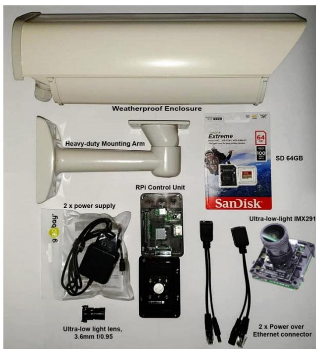
Figure 1 – The components of the RPi camera.
