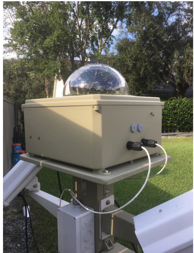
Figure 2 – The 8-camera enclosure on top of a pole that also supports CAMS 230 and CAMS 234.
