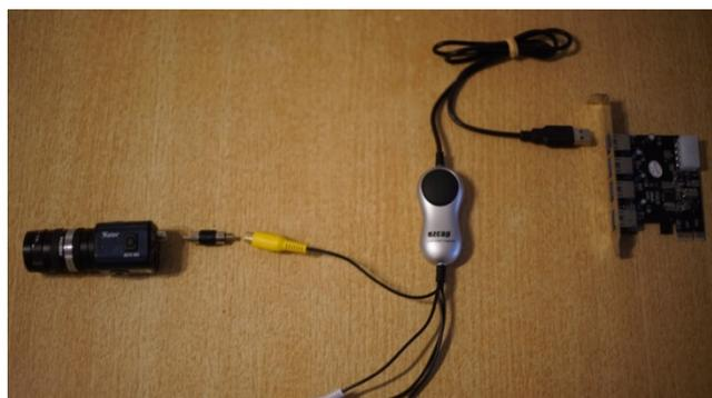
Figure 9 – Typical CAMS hardware configuration.
